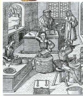
Litho sketch of a German coinery -14th Century - cutting metal pieces, weighing & hammer punching
