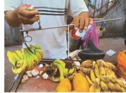
Chinese Market Scale This aluminum balance scale is sold and used widely in China. This scale can be held by larger ring beneath the user right hand to produce leverage for heavier loads
